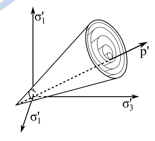
Each homothetic surface is characterised by the backstress tensor defining its centre  $\alpha$  and its opening M (Prevost 1985).
