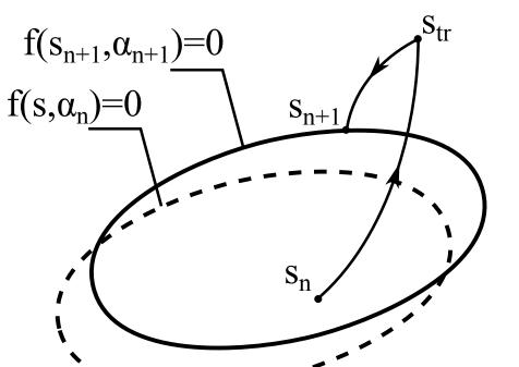
The algorithm is based on a 2-step return mapping
