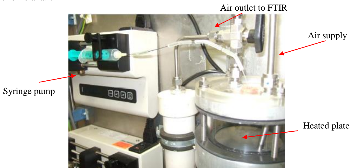
Figure 4.19: syringe pump and heated plate
