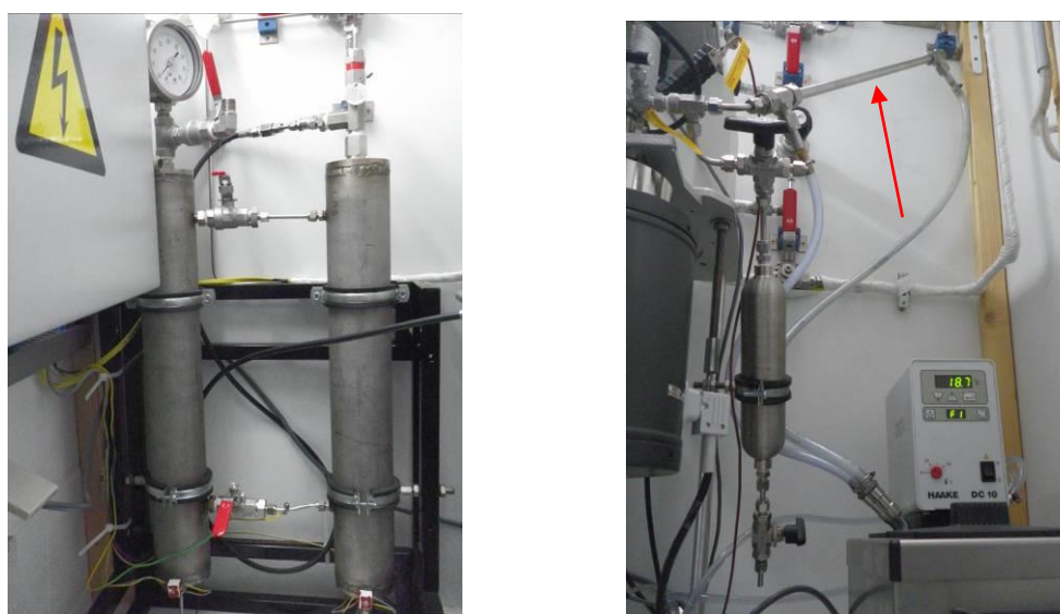
Figure 4.6: Water balance control (saturator and condenser)
