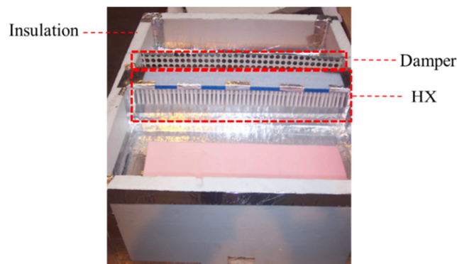
Figure III-36: Box containing the heat exchanger
