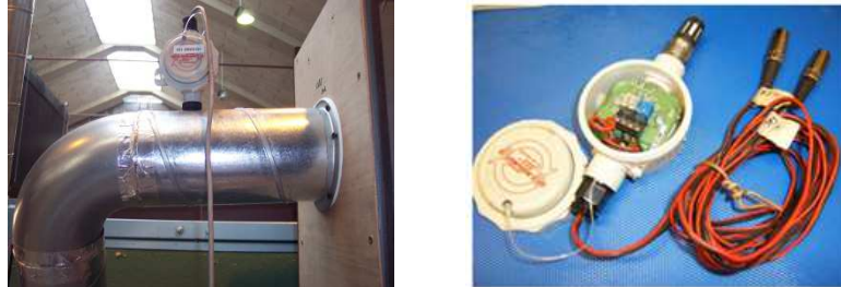
Figure II-18: 'Status instrument' relative humidity sensor
