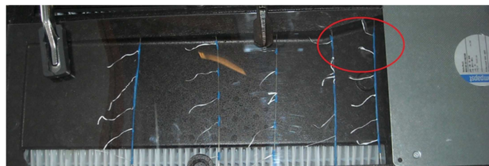
Figure V-22: Area of turbulence at the fresh air fan exhaust
