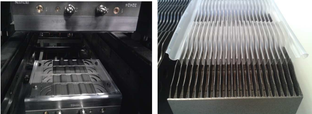
(a) (b) Figure III-29: Thermoforming mold (a) and zoom on the central part of the thermoforming mold (b)
