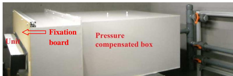
Figure V-15: Insertion of the unit in the pressure compensated box
