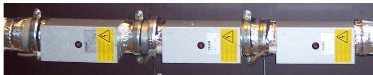
Figure II-16: Resistances of 900W in series
