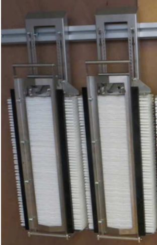
Figure III-32: Press of the heat exchanger
