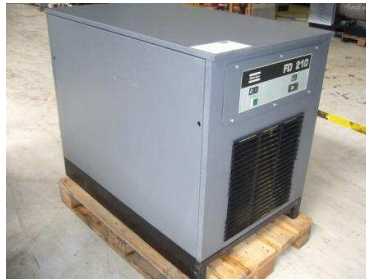
Figure II-15: Industrial air dryer Atlas Copco FD210
