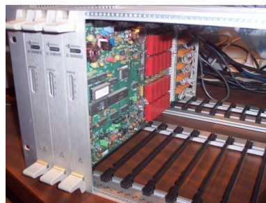
Figure II-20 : Data acquisition cards (Solartron Instruments SI 359551)
