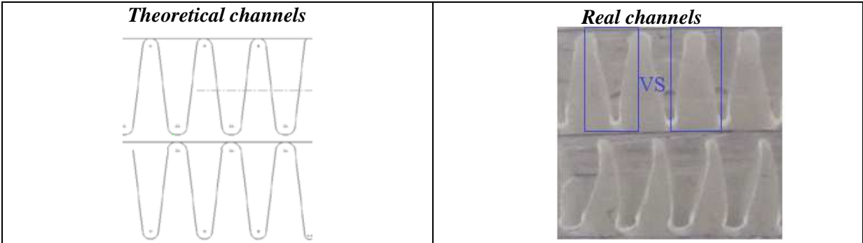
Figure III-42 : Identification of the differences between theoretical and real geometry
