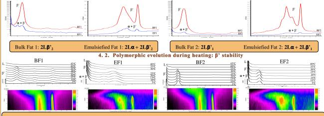
For the emulsified fats, above 25°C, the transition of  $\alpha + \beta$ ' to  $\beta$ ' takes place, due to the melting of  $\alpha$  form. After this no further transitions are being observed until complete transformation to liquid state. The passage to the liquid state takes place without the occurrence of β form, for both fats in both states.
