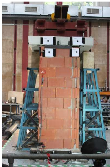
Figure 141 - Position of the slab (L-shaped walls)
