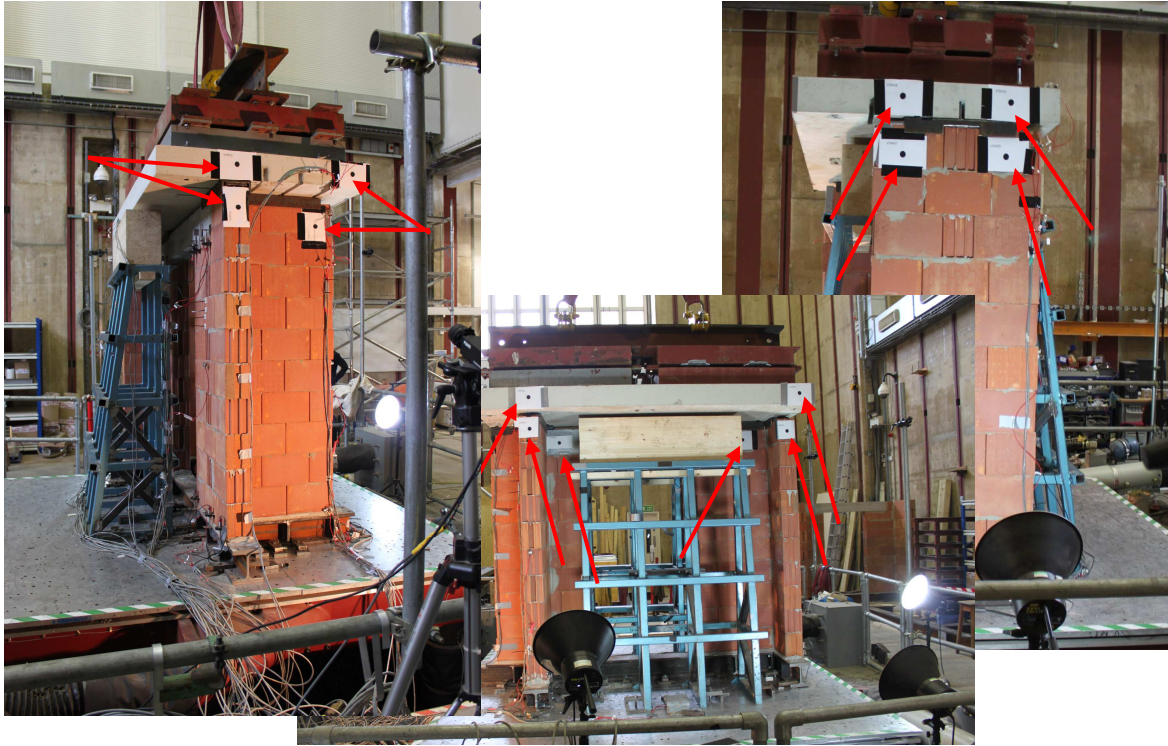
Figure 131 - View of the targets (T-shaped walls) for the Imetrum Video-Gauge Vision System (VS).
