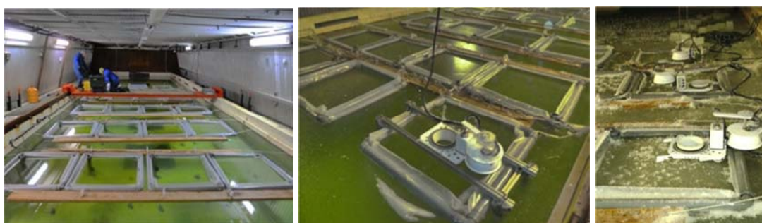
Figure 1. Experimental mesocosms prior to freezing (left). Air-ice CO 2 fluxes measurements over freezing seawater carried out with an automated chamber during freezing (middle) and after the ice had formed to provide solid platform for the chambers (right).
