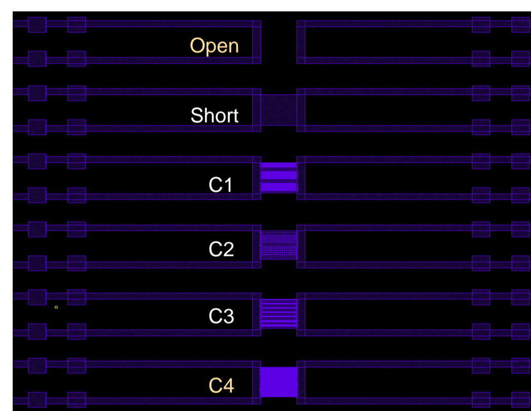
Structure of the chip: 4 different interdigitated electrodes and 2 calibration structures are displayed.
