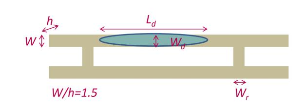
■  $W_r/W < 1 \& L_d > W$  → Droplets can not flow in the rungs
