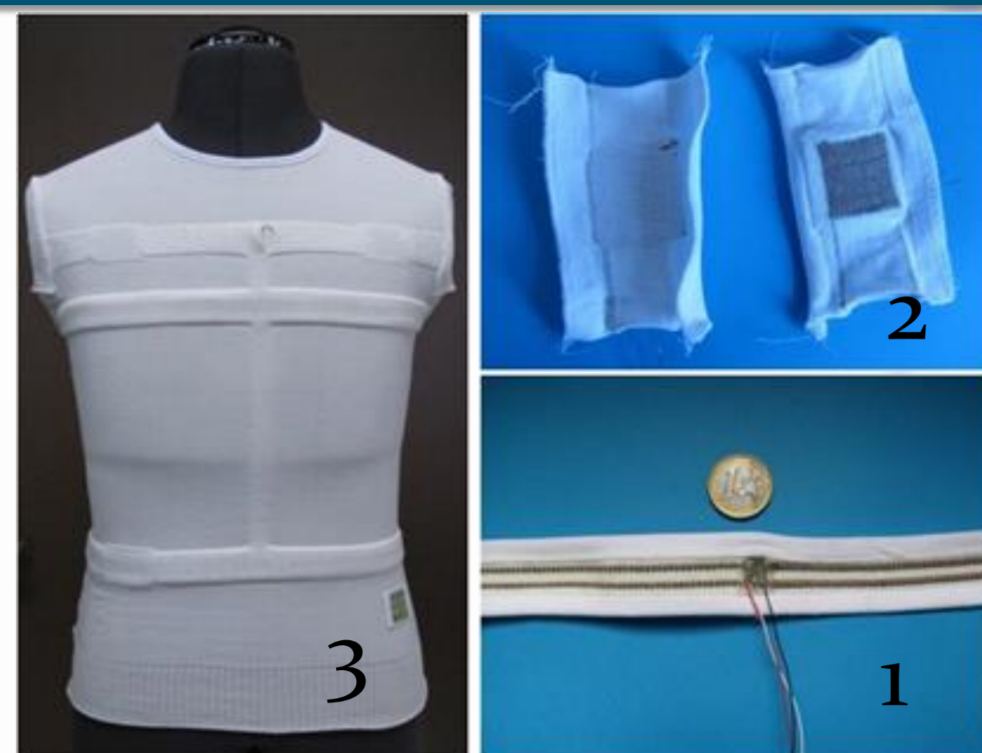
Respiratory belt (1) Electrodes embedded in textile (2) Smart clothes with the integrated respiratory belt (3)
