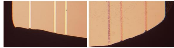
Figure 3: Capture of the partially encapsulated sensor (the encapsulant is in black), Al is not attacked during the test on the sample 4 (left), whereas Al track is attacked on the sample 5 (right).
