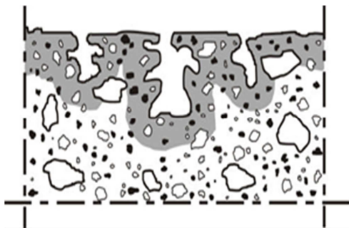
Figure 3. Hydrophobic treatment principle.
