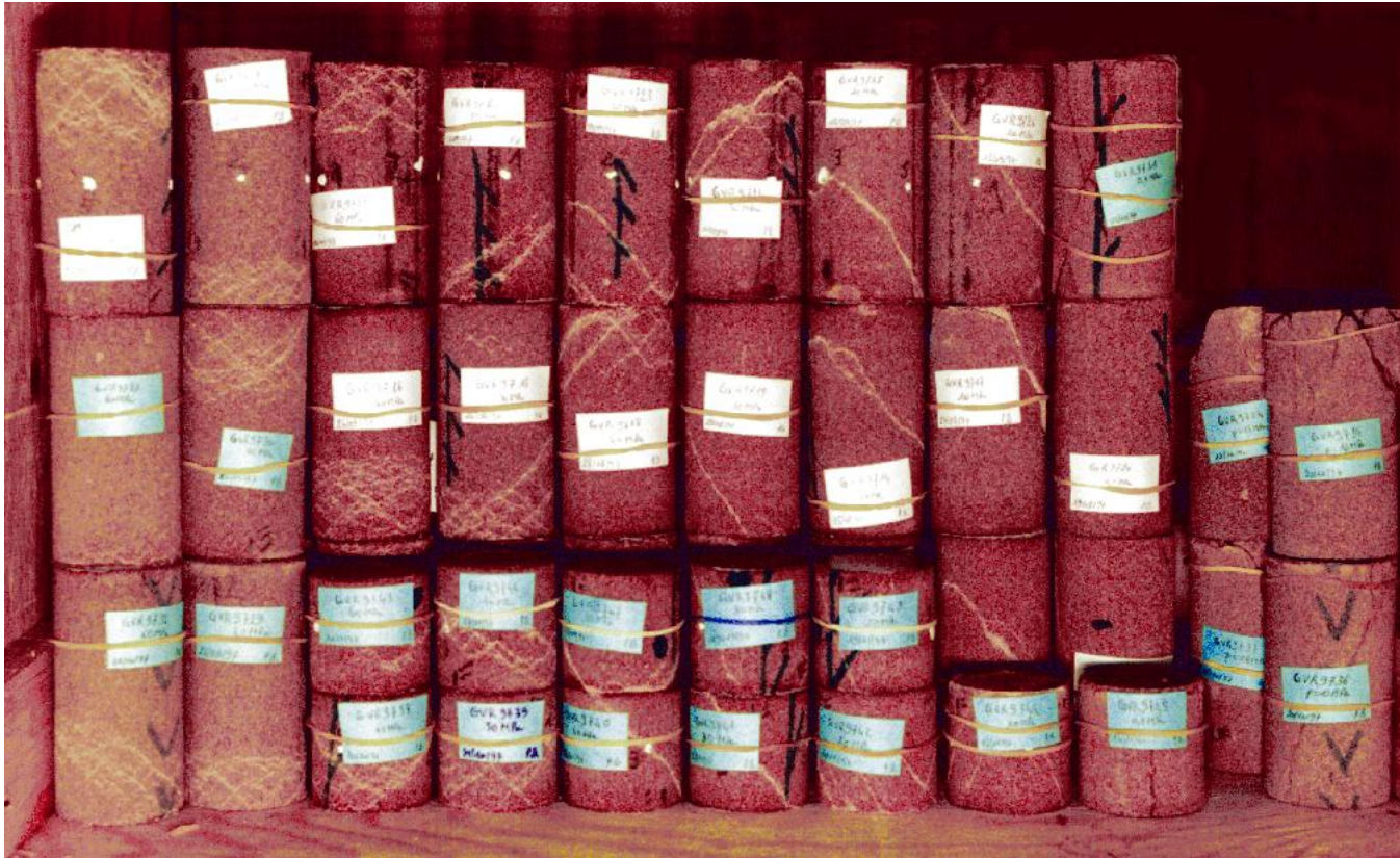
Localized rupture in sandstone samples under different confining pressures (Bésuelle et al., 2000)
