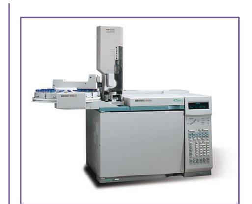
Fatty acid compositions were determined by GC on a HP 6890 Series GC System fitted with a HP 7683 Series injector and flame ionization
