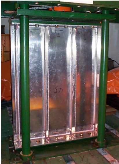
Fig.16(a) Test set-up for physical model testing on stiffened panels (unloaded edges are free)
