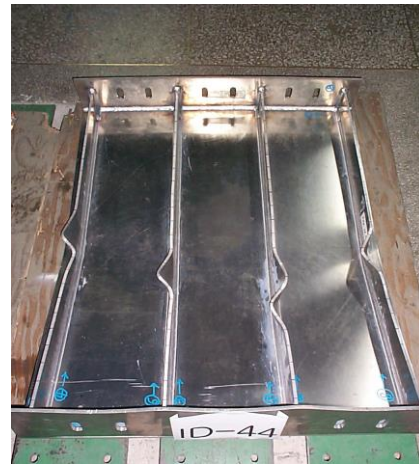
Fig.18(b) A photo of the tested panel failed by stiffener tripping (Mode V) – unloaded edges remain free
