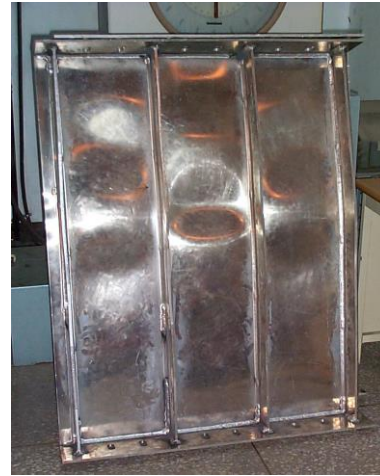
Fig.18(a) A photo of the tested panel failed by beam-column type collapse (Mode III) – unloaded edges remain free
