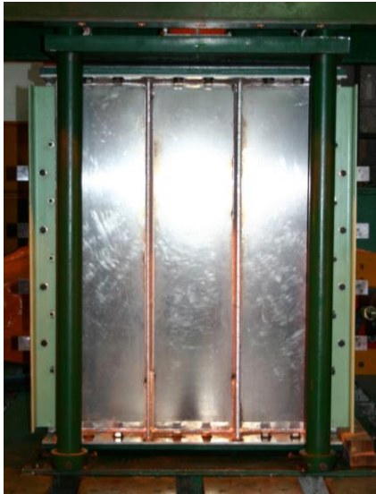
Fig.16(b) Test set-up for physical model testing on stiffened panels (unloaded edges are simply supported and kept straight)
