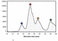
HPSEC chromatograms of hydrolyzed artichoke inulin revealed four peaks. HPAEC-PAD characterization of these peaks permitted the identification of fructose, F<sub>2</sub>, F<sub>3</sub> and F<sub>4</sub>. HPSEC provided sufficiently good separation of extracted Fn as some relatively pure fractions were obtained for mass spectrometry characterization.
