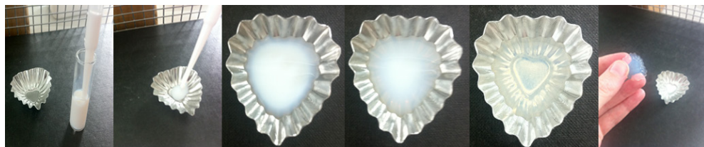
Figure 1. The visible process by which the polymer liquid solidifies to form a cross-linked hydrogel
