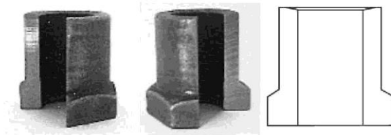
Fig. 8. Collar 16 mm diameter: actual and modelled shapes.
