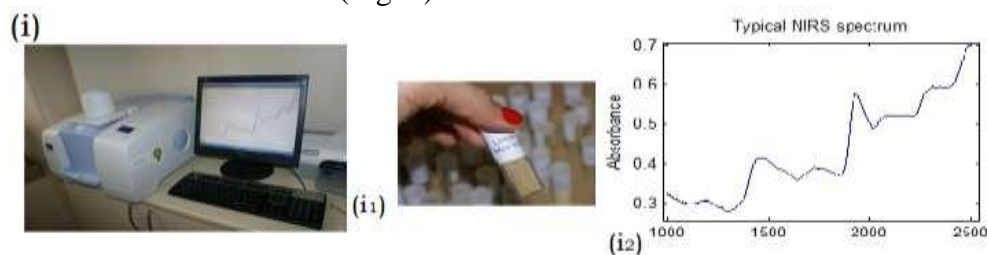
Figure 1. Acquisition of spectrum/spectra by conventional NIR spectroscopy system (source USAMV Cluj, Romania)
