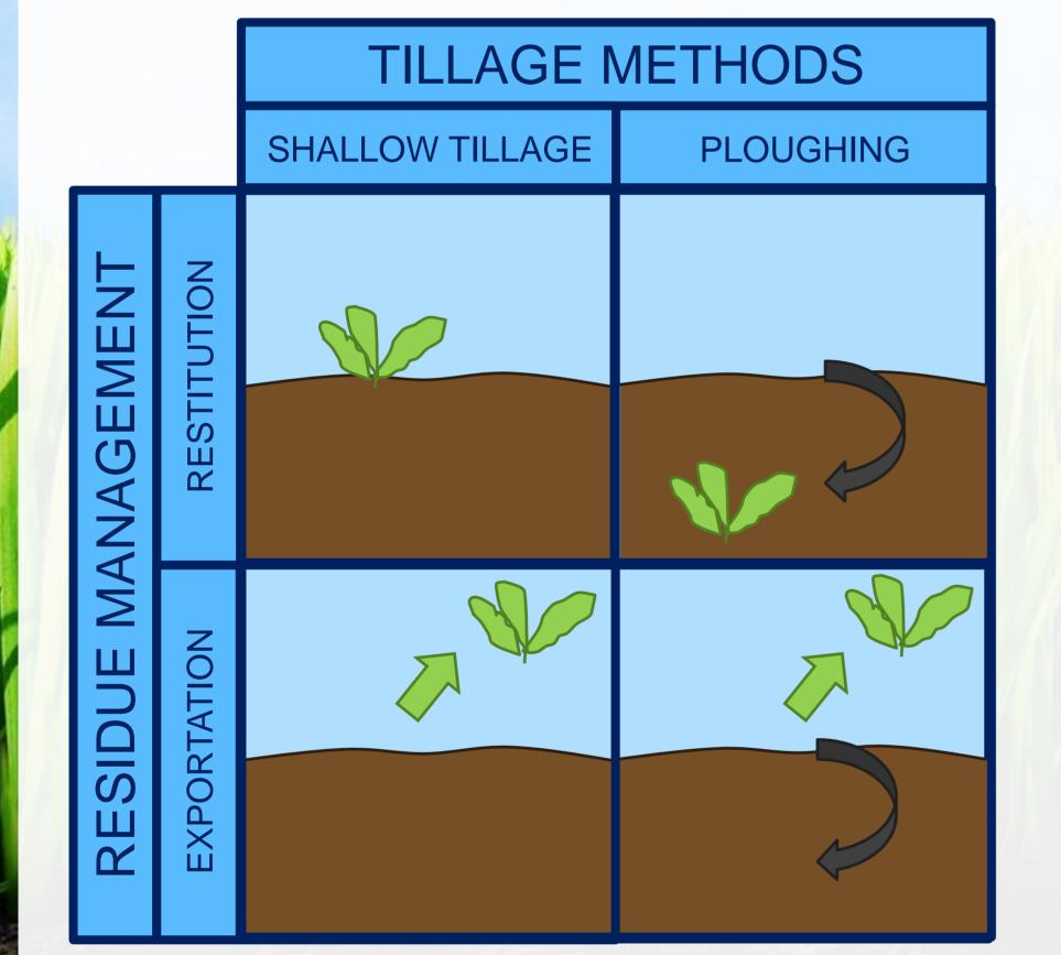
Four modalities are tested in relation to the destiny of crop residues whether they are exported or not and the tillage methods whether the field is ploughed or shallow tilled.
