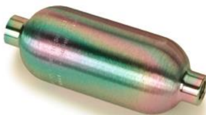
Figure 2.11: cylinder for thermal degradation with CO 2
