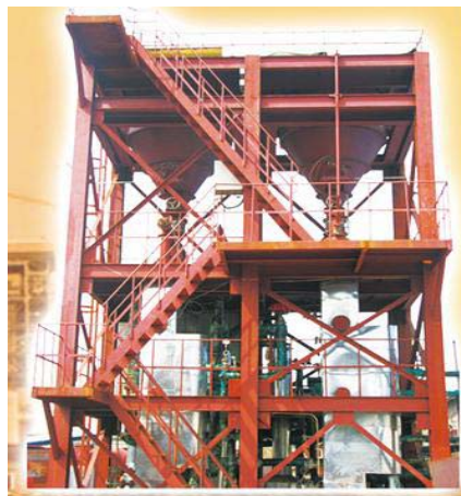
Figure 5. Pilot-scale testing system of lignite drying.
