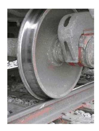
Vibrations and noise are generated as rough wheels roll over rough supports.
