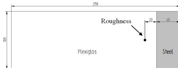
Figure 2. Top view schematic of the flat plate for H3 testing
