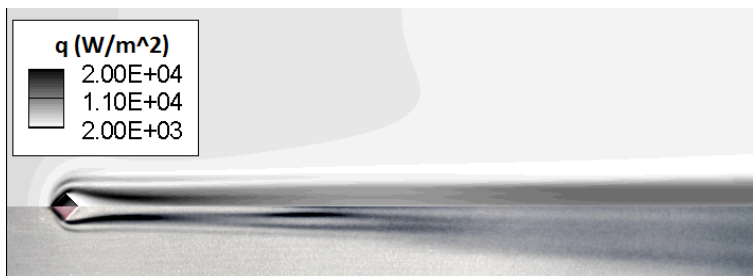
Figure 23. Heat flux experimental(bottom)-numerical(top) distributions comparison : square
