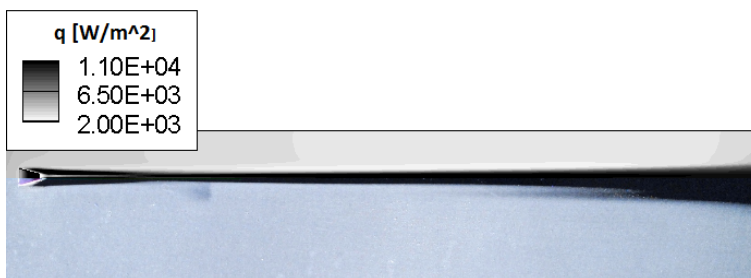
Figure 15. Heat flux experimental(bottom)-numerical(top) distributions comparison
