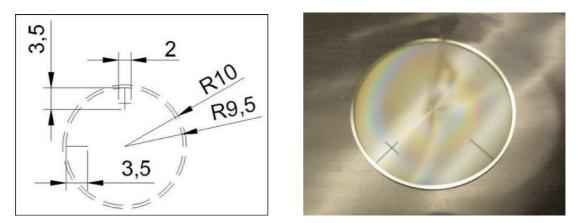
Figure 6. Left: Schematic diagram of the fiducials used for centering the AGPM. Right: Lines (centering marks) deposited by AJP on the VISIR-AGPM coronagraph.
