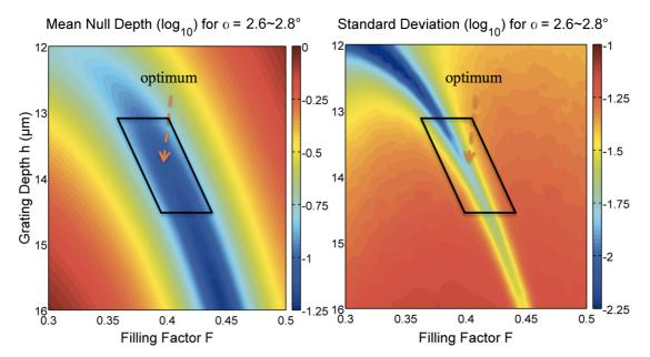
Figure 3. RCWA multi-parametric simulation: mean (left) and standard deviation (right) of the Mean Null Depth (logarithmic scale) over the upper N-band, with  $\alpha$  ranging from 2.6 to 2.8°. The period is set to  $\Lambda = 4.6 \ \mu m$  (SWG limit).
