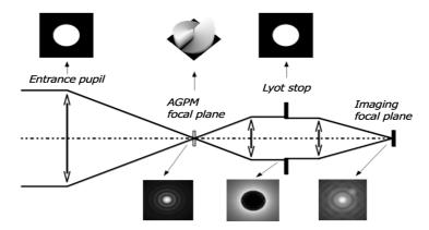
**Figure 2.** AGPM coronagraphic optical bench scheme. Numerical coronagraphic simulation illustrating the diffractive behavior of the AGPM in the *K*-band (Mawet *et al.* 2005<sup>1</sup>).
