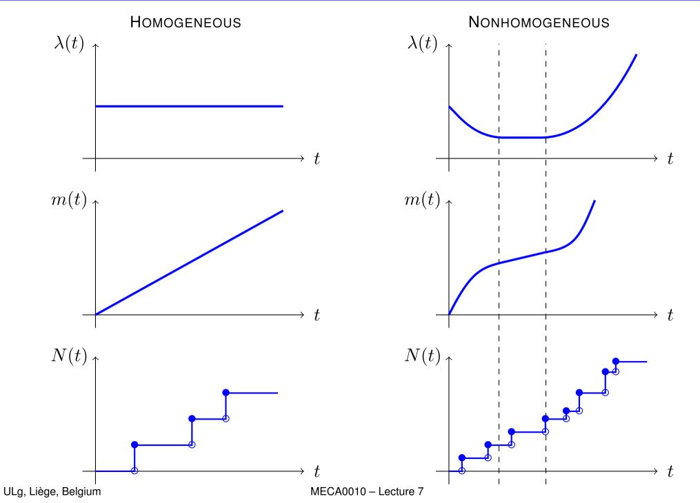
For a nonhomogeneous Poisson process  $\{N(t), t \ge 0\}$  with (instantaneous) intensity  $\lambda$ , the first time to failure  $T_1$  admits as a probability density function
