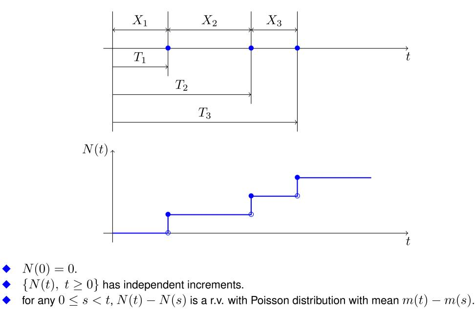
The Poisson process  $\{N(t), t \ge 0\}$  is **homogeneous** if the mean function m is of the form  $m(t) = \lambda t$  with  $\lambda$  a positive constant, that is, if the average number of failures occurring increases linearly with the time interval under consideration.
