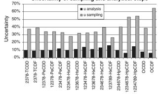
Fig. 3 Uncertainty of the sampling and analytical steps of the method
