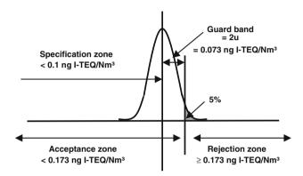
Fig. 5 Guard band for the decision-making process
