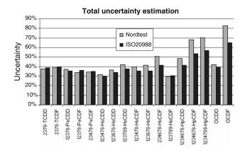
Fig. 1 Nordtest versus ISO 20988 results for the period 2002-2007
