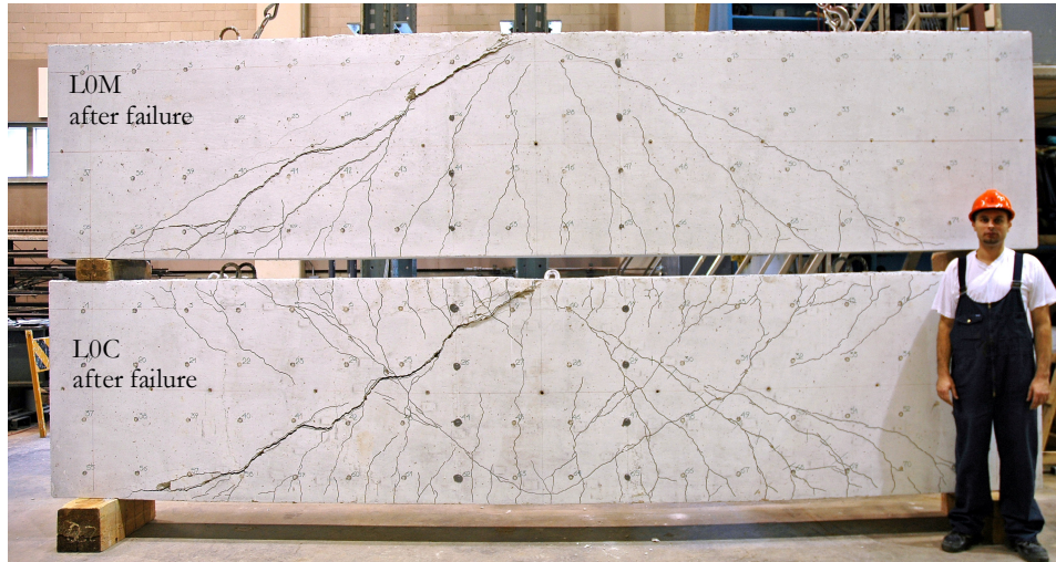
Figure 4.34 Specimens L0M and L0C after failure
