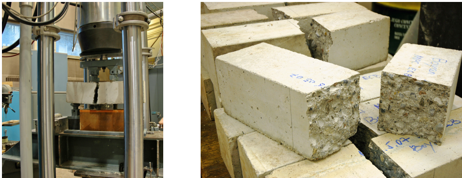
Figure 3.8 Modulus of rupture test – specimens SB and MB
