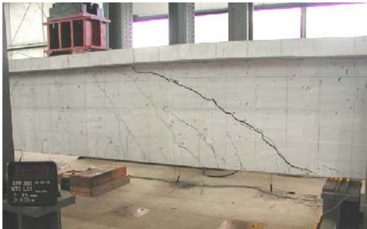
Figure 5.5 Failure of specimen 01T0 tested by Higgins et al. (2004)
