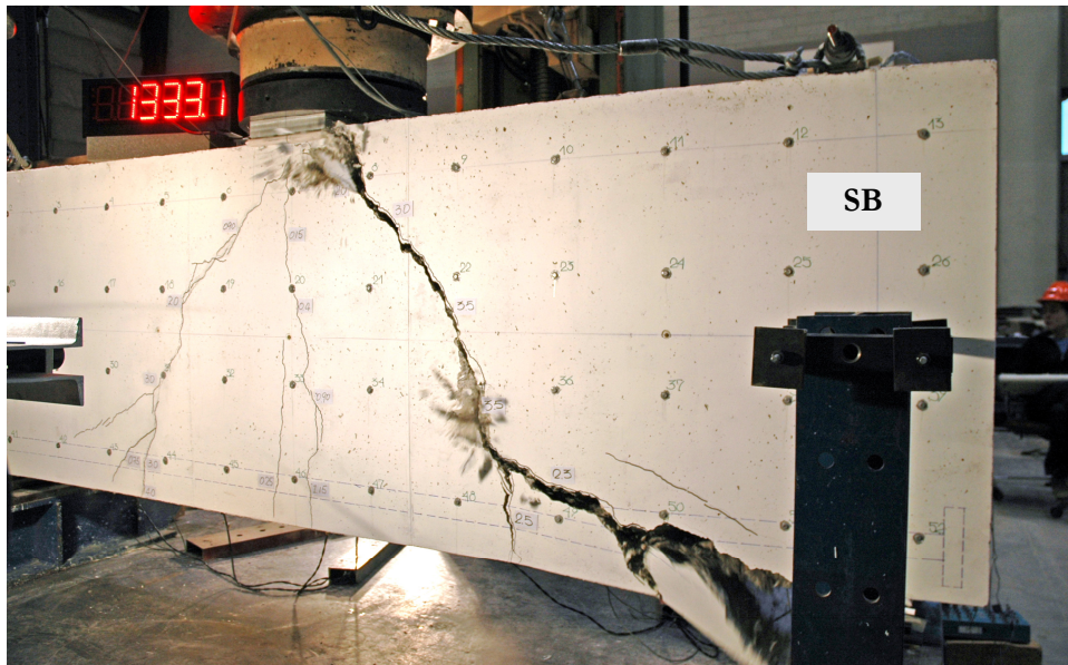
Figure 4.54 Failure – specimens MB and SB
