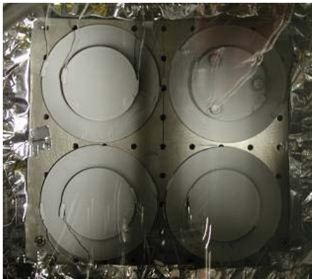
Fig. 6: Integration of the SiC/SiC samples in the vacuum chamber
