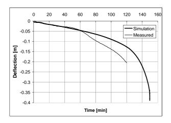
Fig. 9. Deflection of the secondary edge beam
