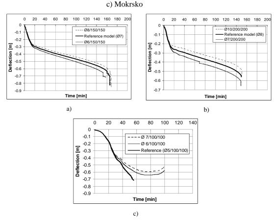
Fig. 17. Influence of the reinforcement: a) FRACOF b) COSSFIRE c) Mokrsko
