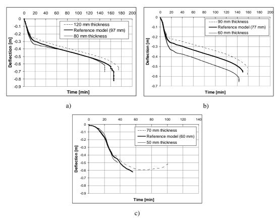
Fig. 16. Influence of the slab thickness: a) FRACOF b) COSSFIRE
