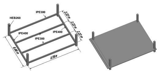
Fig. 1. Tested structure (Zhao et al., 2008)
