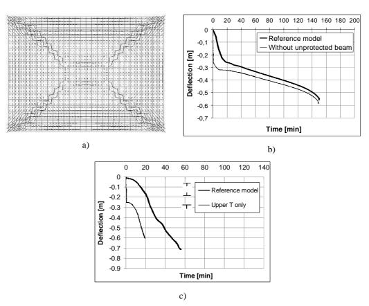
Fig. 15 Presence of the unprotected beam: a) FRACOF b) COSSFIRE c) Mokrsko
