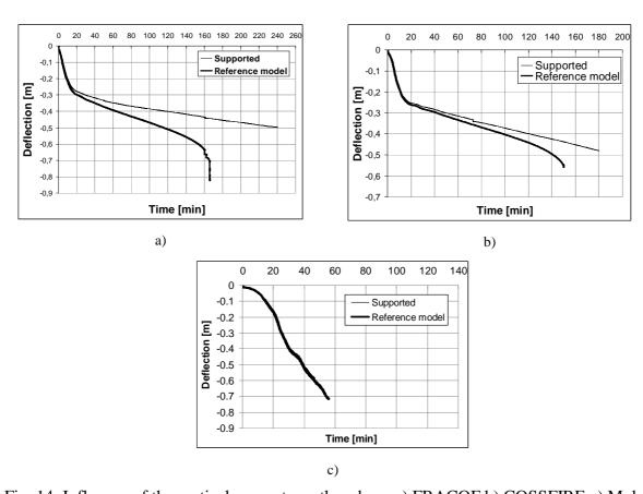
Fig. 14. Influence of the vertical supports on the edges: a) FRACOF b) COSSFIRE c) Mokrsko
