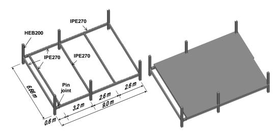
Fig. 5 Tested structure (COSSFIRE, 2006)
