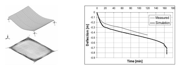
Fig. 4 Deformed shape and membrane forces – Deflection in the middle of the slab
