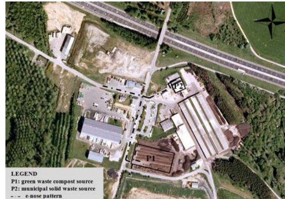
Figure 1: Identification of odour sources of the waste treatment plant investigated and e-nose pattern
