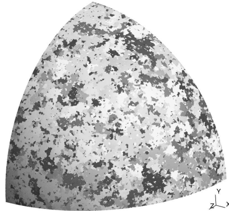
Figure 5.20: Final configuration of the fragmentation of a sphere with a strain rate of 1e^4 [s^{-1}] .
