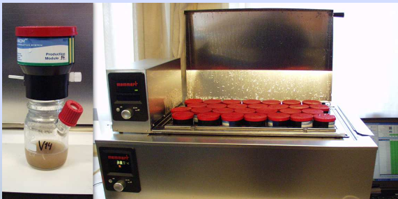
Figure 1a. Glass bottle equipped with a pressure sensor module (Gas Production System, Ankorm RF). Figure 1b. Fermentation during 72h at 39°C in a shaking water-bath.
