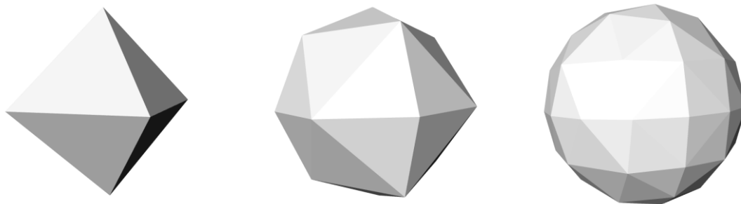
Figure 4: Generation of the set of directions examined for the rose diagram. The method begin with an octahedron (left) and iteratively subdivides the edges and projects the generated vertices onto a sphere, obtaining 18 vertices at step 1 (centre), 66 vertices at step 2 (right), etc.
