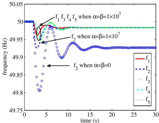
**Notes:** (i) Frequency deviations in area 2 are much smaller in the presence of the control scheme. (ii) All the frequencies converge towards the same value under the control scheme. (iii) Voltage excursions in the DC grid are small (less than 1%).
